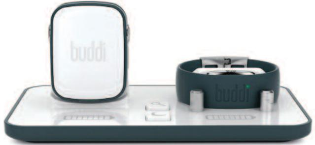
**Key features:** GPS tracking; two-way voice communication with monitoring centre; geofence capability; geofence safe and unsafe zones; manual alarm button; fall detection; online access; email and text-message notifications.
